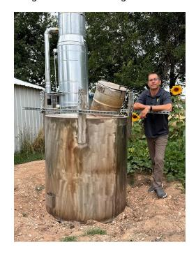
burn pit or a Kon Tiki, making the process better both for the user and the environment. Having the pit covered also allows for a full cool down after quenching rather than having to dig out the biochar while it is still warm. This stove was designed with the global south in mind. It allows for large volumes of biochar to be created but with less risk. This is a very versatile design that can be altered to fit the feedstock and location needs with minimal changes.
